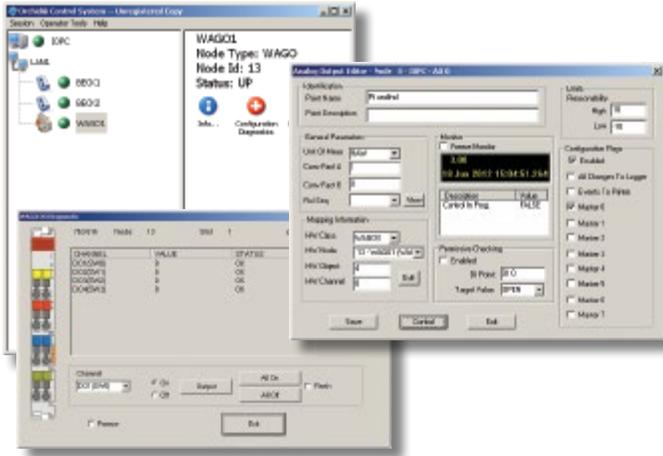
**Orchid® IO software provides all the features necessary to configure, monitor and troubleshoot the I/O system from any computer on the I/O network**
