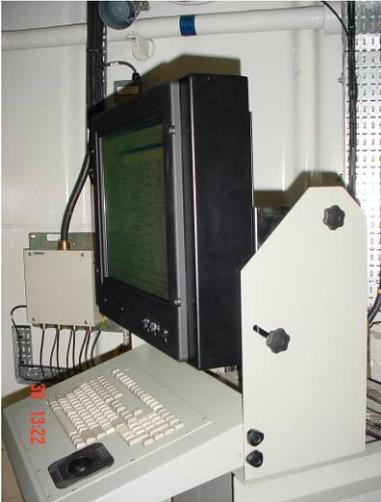
DSAC LCD Screen mounting arrangement
