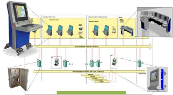
**Figure 1: Typical IPMS Configuration**
